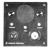
Recess for extra instrument (diam, 52 mm = 2") covered with dummy plug.
